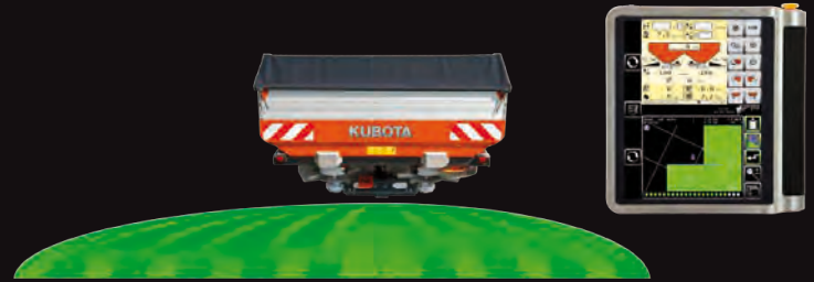
Decreasing the spreading width on the right hand side by 6m
