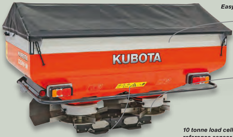
Three options of hopper capacity 1,100 – 1,550 – 2,000 litres
